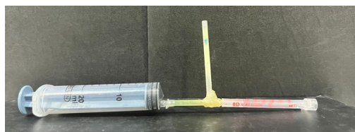
Conventional volume potometer vs Innovative student version
