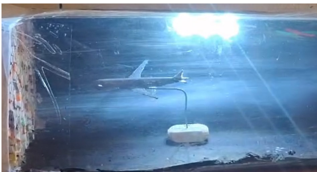
Shyam - Wind tunnel experiment, produces a controlled stream of air to test the aerodynamic characteristics of objects
