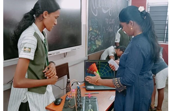
Neha R - An Arduino Uno-based radar system detecting objects by sending signals and analyzing reflections, commonly used for distance measurement and motion detection.
